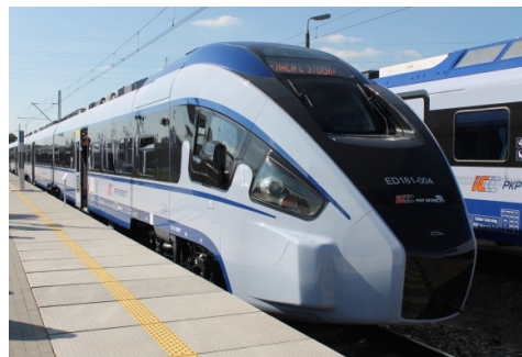
Fig. 2. The most recent train made by PESA, DART, which operates in Poland with maximum speed 160 km/h (optional 250 km/h), [3]
